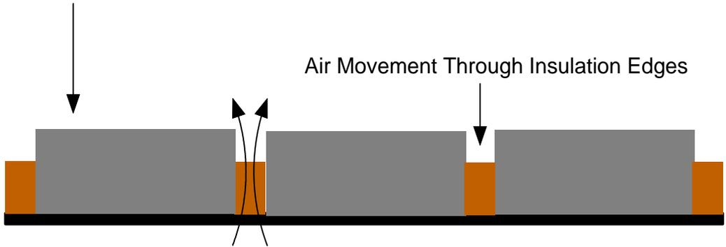
Heat Loss Through Joist And Small Gaps Can Reduce Performance By 28% to 50%
