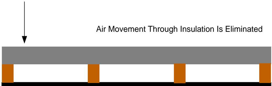
Heat Loss Through Joist Are Eliminated And Can Increase Performance By 48%
