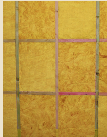
Properly fitted wall insulation in test with no gaps around the edges of the insulation.
