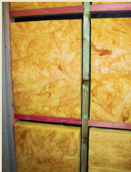
Wall in test with larger gaps around the edges of the insulation.
